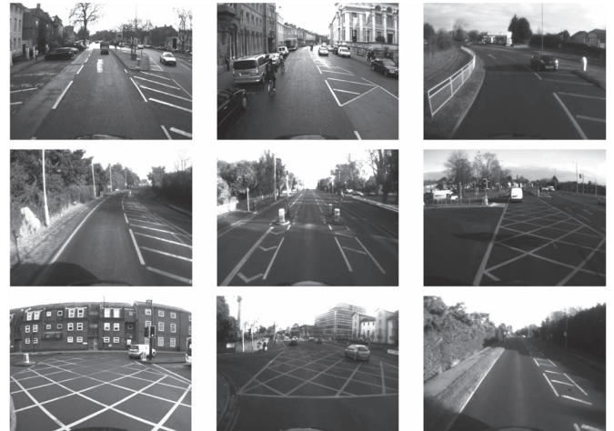
Fig. 12. Examples of boxed junctions correctly classified by our algorithm (86% prediction accuracy). Thus no stopping or traversal areas are automatically detected.
