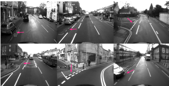
Fig. 6. Special lane and intersection type road markings have very similar visual appearance (short, repetitive).
