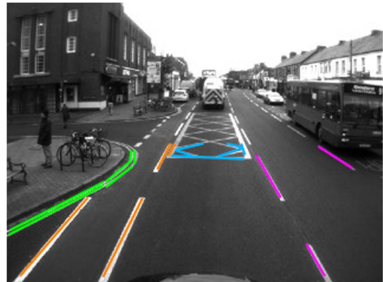
Fig. 1. Reading the road requires classifying and interpreting the meaning of road markings in the road scene. Here, each colour represents a unique road marking class.
