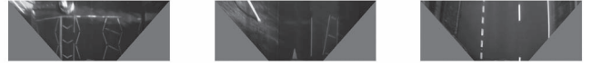
Fig. 3. Inverse Perspective Mapping (IPM) to remove the perspective effect in images. Notice how, in the IPM images, parallel lines no longer intersect at the vanishing point. Thus true lengths, orientations and positions can be recovered.
