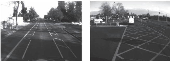
Fig. 7. Boxed junctions describe areas of the road that a vehicle should not be stationary in (but may possibly quickly traverse) such as separator boxed junctions (left) and intersection boxed junctions (right).
