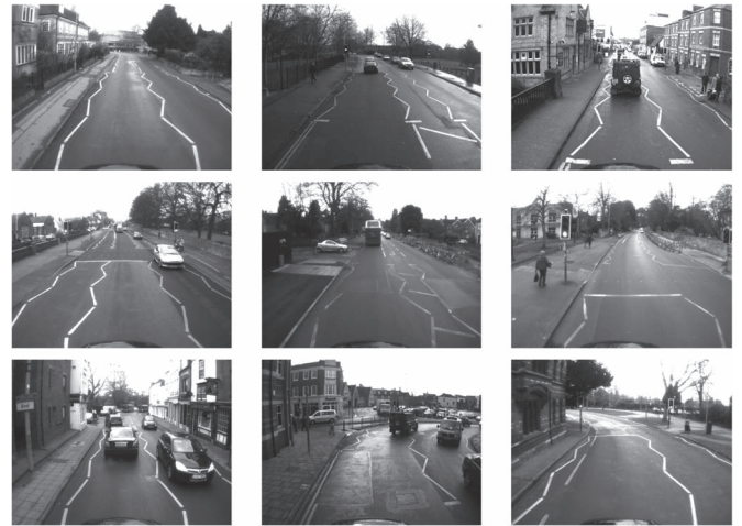
Fig. 11. Some zig-zag approaches correctly classified by our algorithm, with 88% accuracy. Thus our vehicle can anticipate upcoming traffic light controlled pedestrian crossings.
